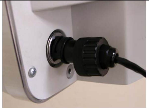
ODU connection not weather secured
