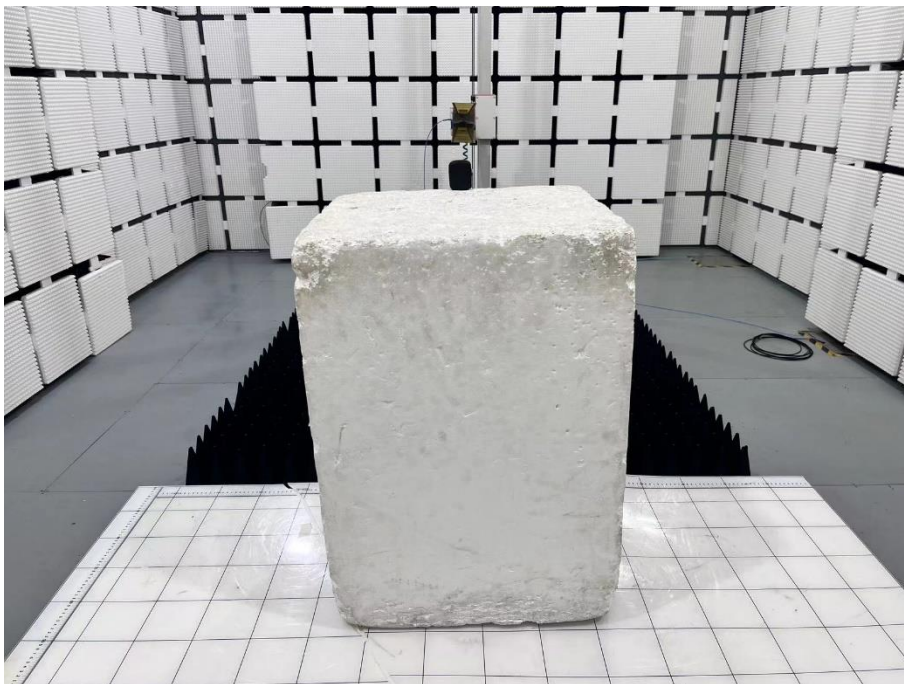
Set-up for Radiated Spurious Emission, Above 1GHz
