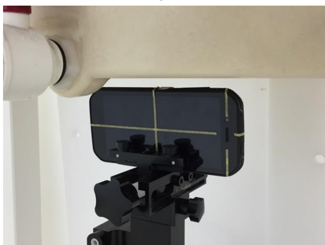
Left Side, Test Separation 10 mm
