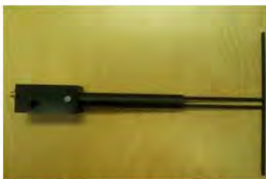
Figure 1 – MVG COMOSAR Validation Dipole
