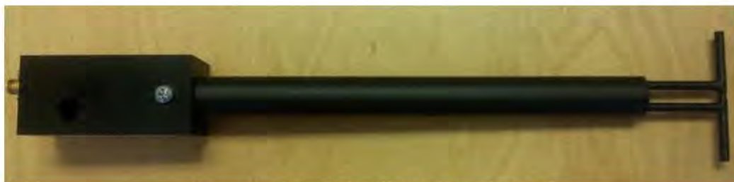
Figure 1 – MVG COMOSAR Validation Dipole
