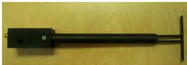
Figure 1 – MVG COMOSAR Validation Dipole
