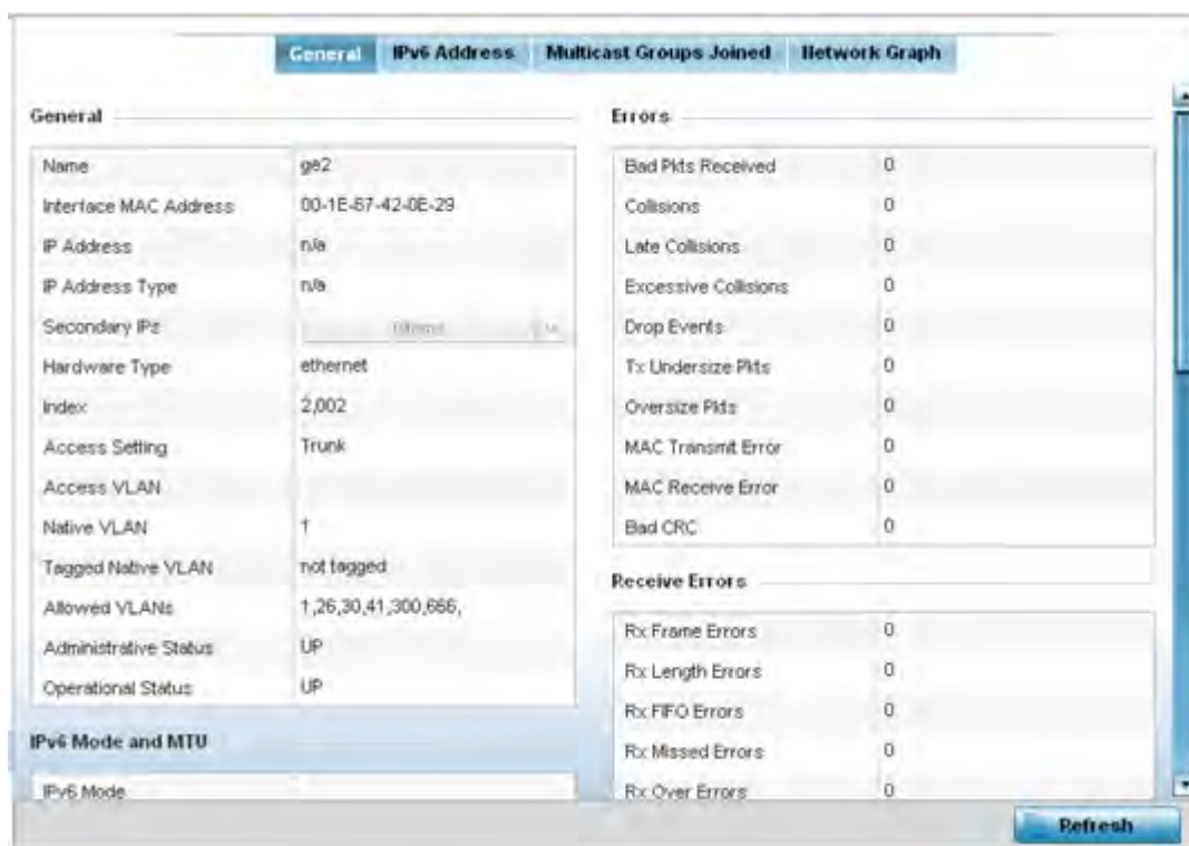
Figure 15-58 Wireless Controller - General Interface screen
