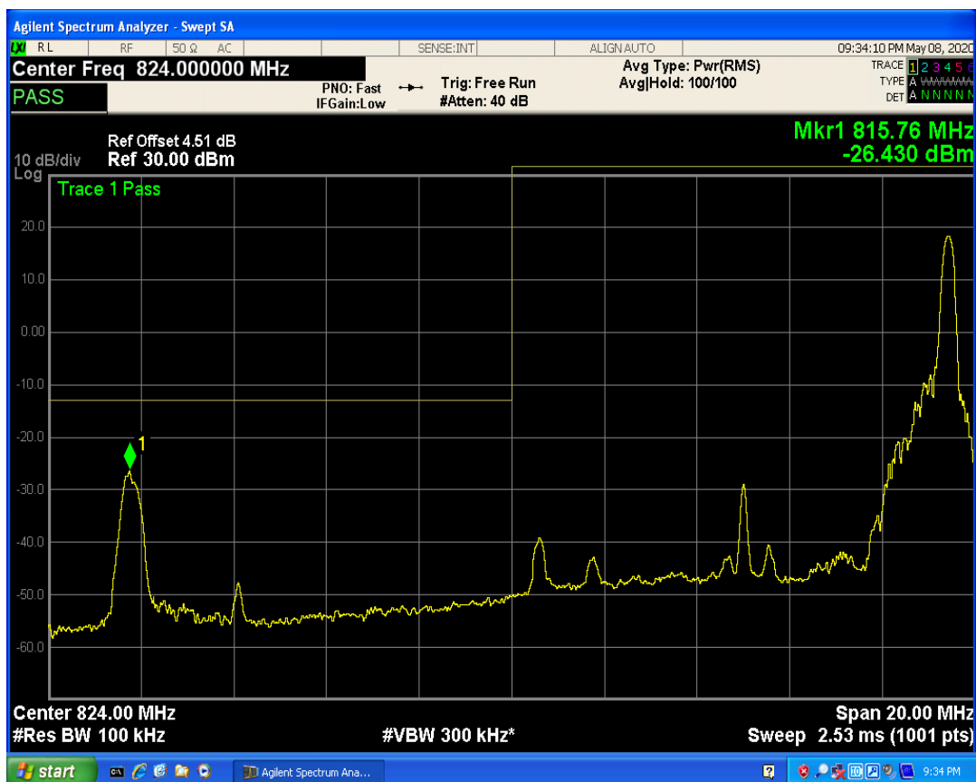
LTE Band5 QAM16 BW=10MHz Channel=20450 RB Size=50 Position=#0
