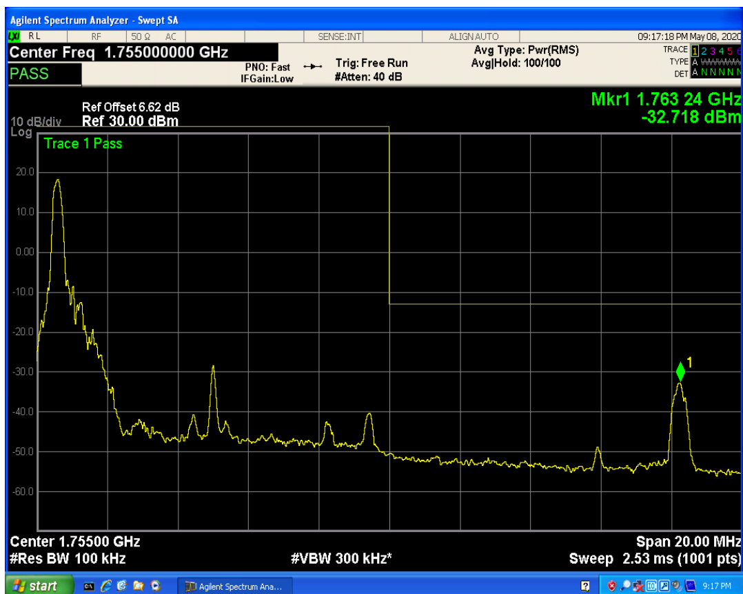
LTE Band4 QAM16 BW=10MHz Channel=20350 RB Size=1 Position=#Max
