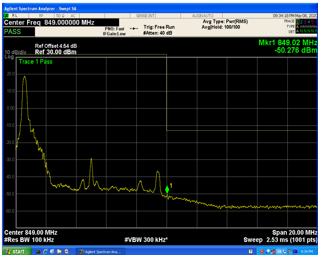
LTE Band5 QAM16 BW=10MHz Channel=20600 RB Size=1 Position=#Max
