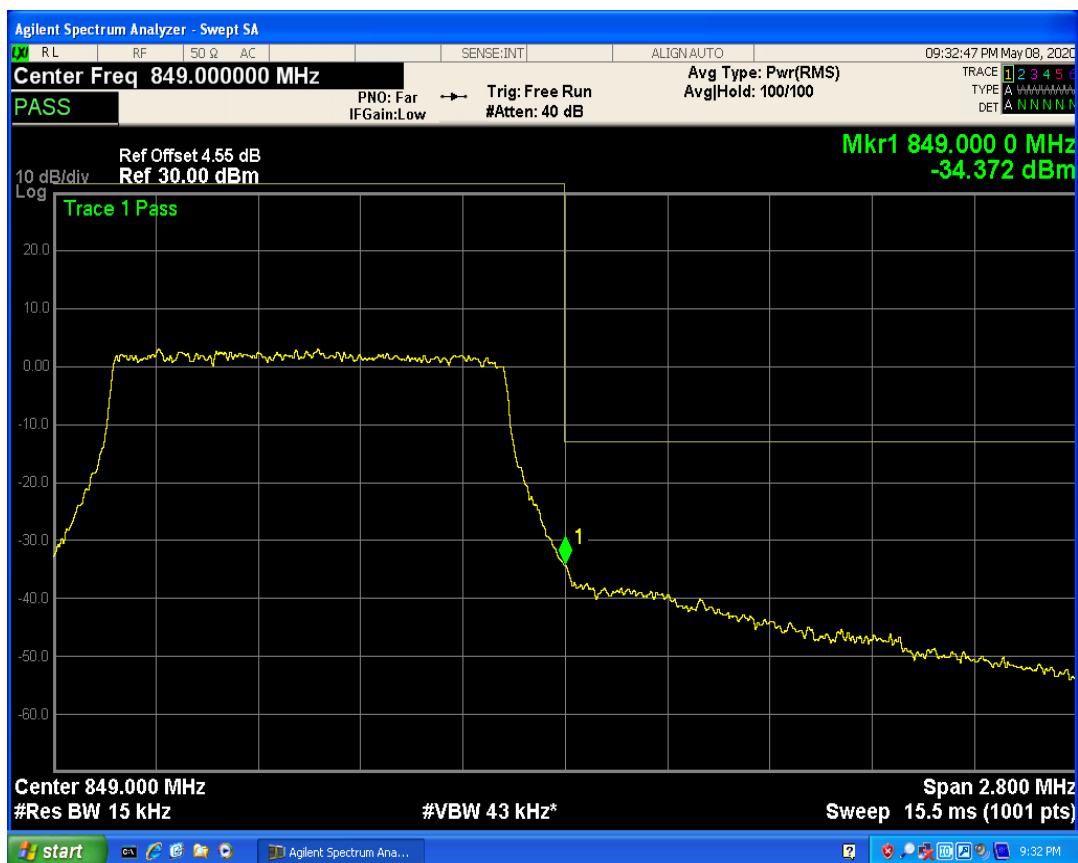
LTE Band5 QAM16 BW=3MHz Channel=20415 RB Size=1 Position=#0
