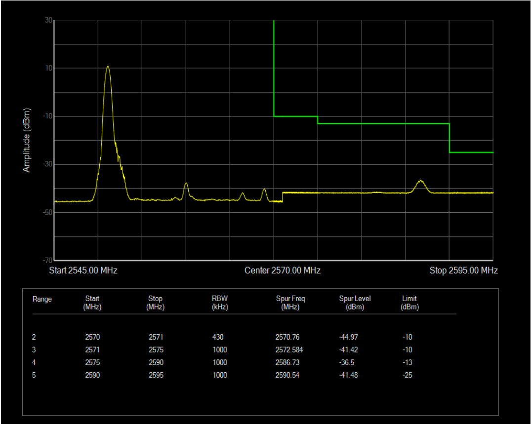
LTE Band7 QAM16 BW=20MHz Channel=20850 RB Size=100 Position=#0
