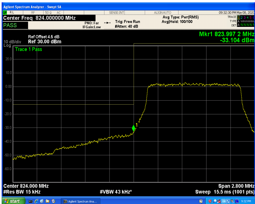
LTE Band5 QAM16 BW=1.4MHz Channel=20643 RB Size=1 Position=#Max
