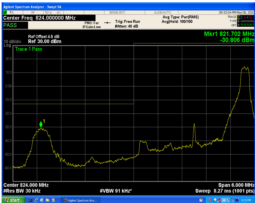
LTE Band5 QAM16 BW=3MHz Channel=20635 RB Size=1 Position=#0
