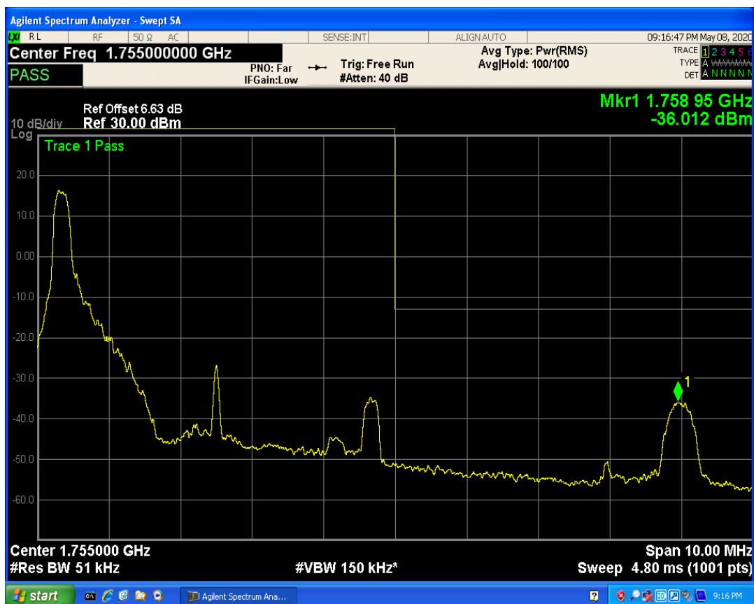
LTE Band4 QAM16 BW=5MHz Channel=20375 RB Size=1 Position=#Max
