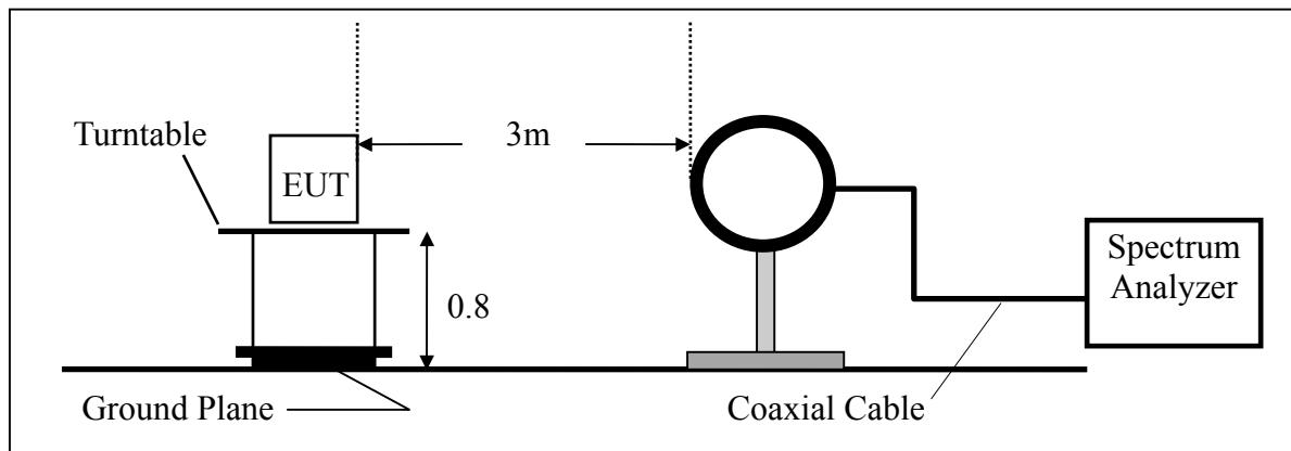
**For Frequencies below 1 GHz**
