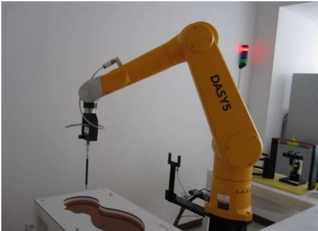
Picture C.1: Specific Absorption Rate Test Layout
