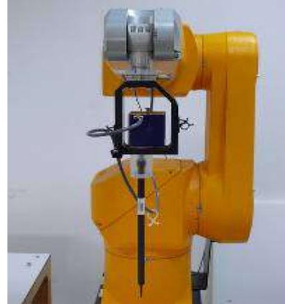
Figure 5-3. ES3DV3 E-field probe
