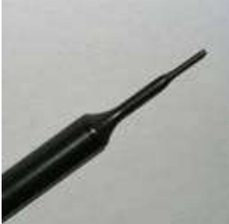
Figure 5-2.ES3DV3 E-field Probe
