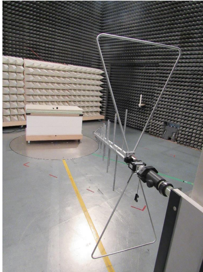
Setup 30 MHz to 1 GHz measurements B
