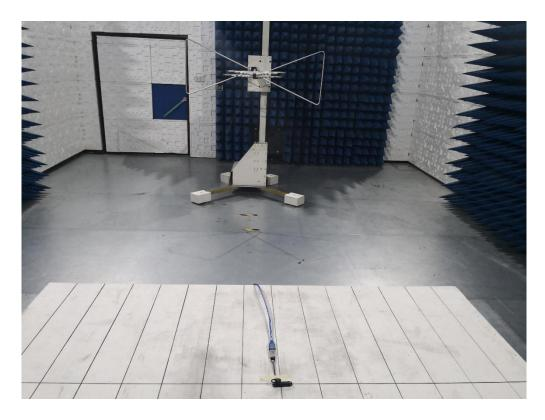
RADIATED EMISSION TEST SETUP ABOVE 1GHZ
