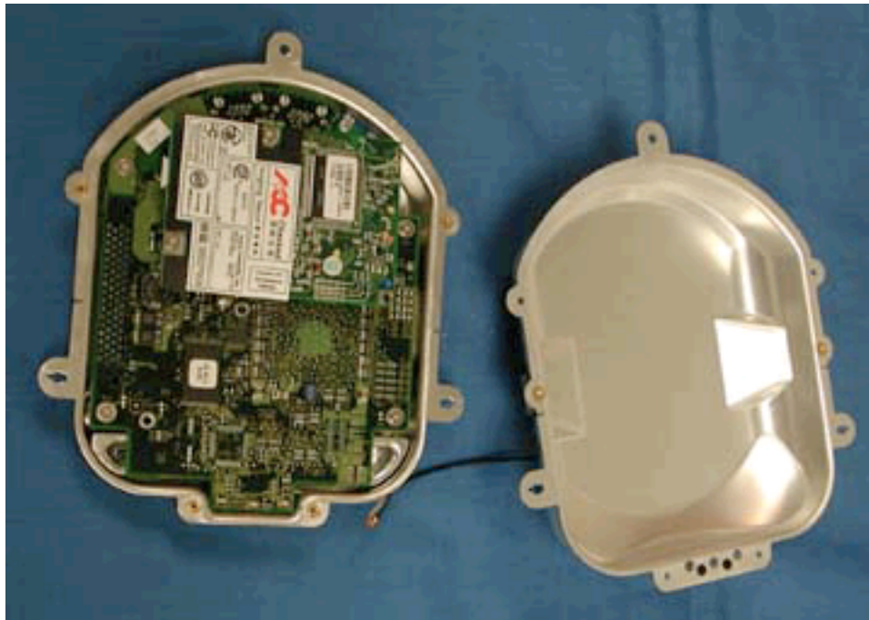
Photo 6 Apple Airport Base Station - Metal Enclosure Cover Removed
