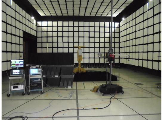
Radiated Spurious Setup for 40-100 GHz
