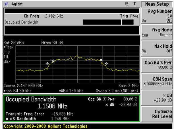
20dB Bandwidth plot on channel 39 (1Mbps)
