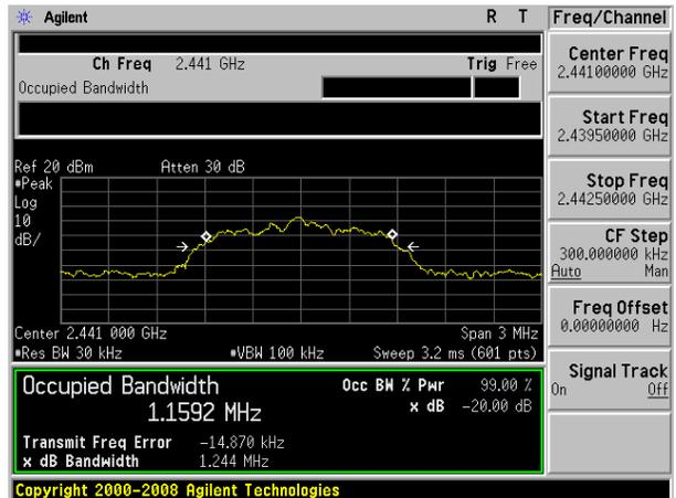
20dB Bandwidth plot on channel 78 (1Mbps)
