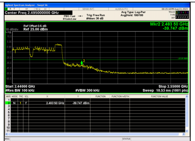
Out Of Band Emission IEEE 802.11ax_Channel 9_40MHz_Antenna 0_RU&Index 52RU44
