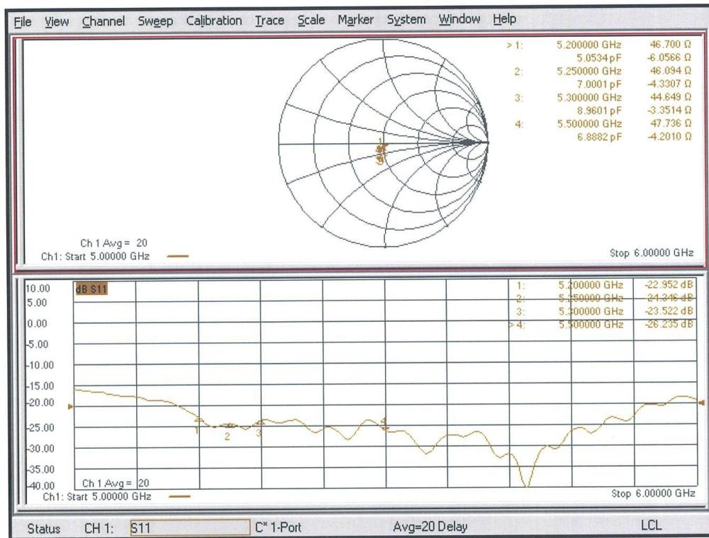
Impedance Measurement Plot for Head TSL (5600/5750/5800MHz)
