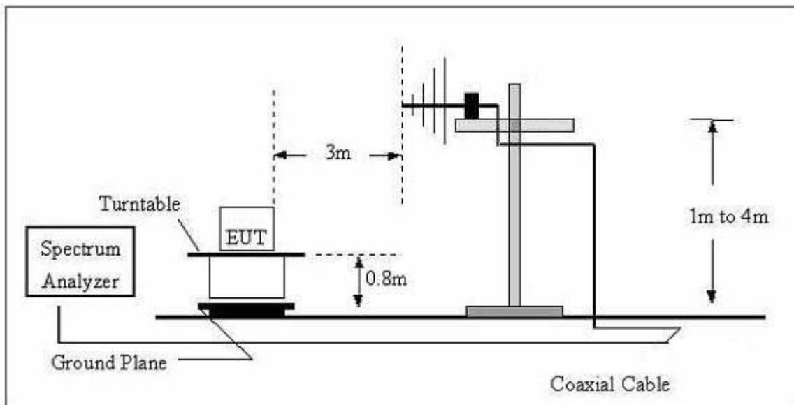
(C) For radiated emissions above 1000MHz
