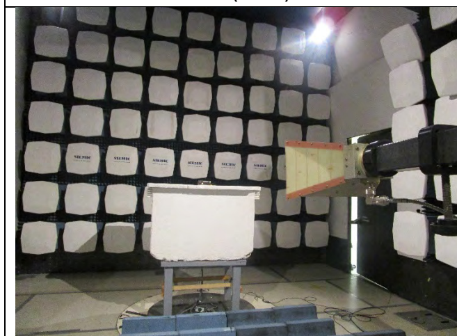
Radiated Emissions (>1GHz) – Front View
