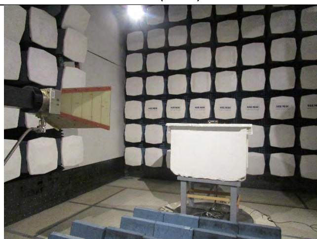
Radiated Emissions (>1GHz) – Rear View
