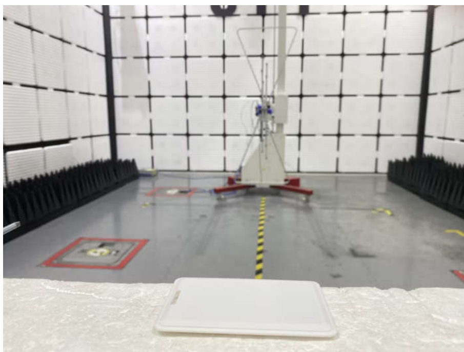
Radiated spurious emission Test Setup-2(Below 1GHz)Close up photo
