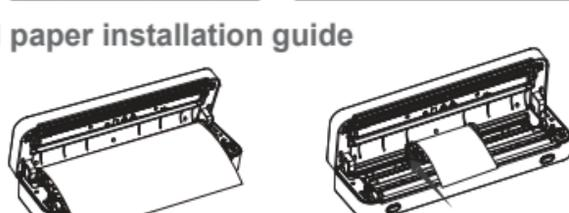
Note: 1. The end of the paper needs to be exposed to the machine. 2. Rolls of different sizes can be fixed by pushing the paper limiter to the edge of the roll when installing different sizes of rolled paper.
