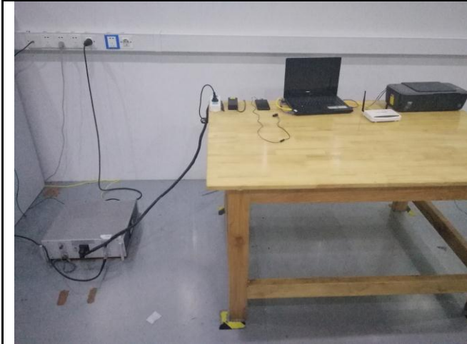
Conducted Emissions Test Setup – Front View
