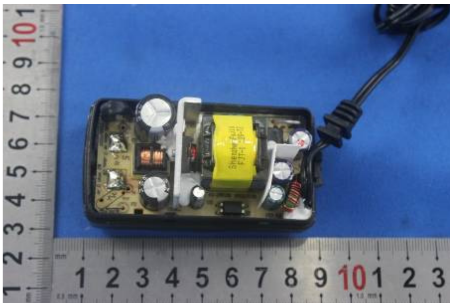
Power supply unit (model No.: FJ-SW1301000N) Internal view
