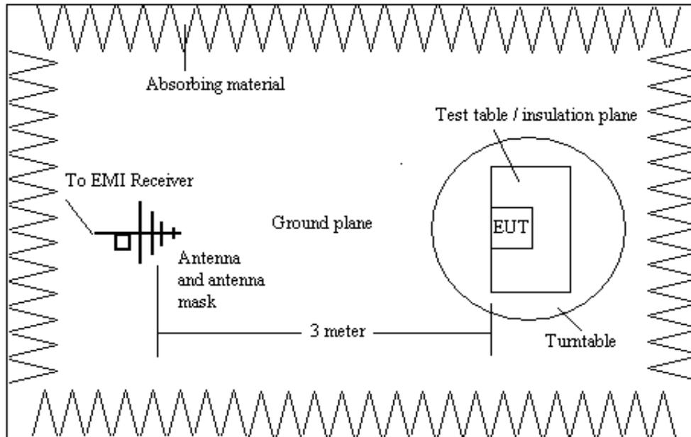
1. For below 1GHz, the EUT was placed on the top of a rotating table 0.8 meters above the ground at a 3 meter semi-anechoic chamber. The table was rotated 360 degrees to determine the position of the highest radiation.
