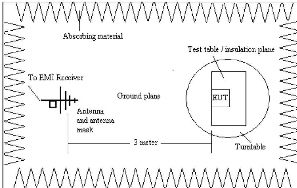
1. For above 1GHz, the EUT was placed on the top of a rotating table 1.5 meters above the ground at a 3 meter semi-anechoic chamber. The table was rotated 360 degrees to determine the position of the highest radiation.
