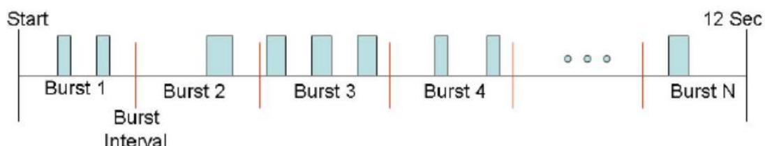
**Table D.7: Frequency Hopping Radar Test Waveform**
