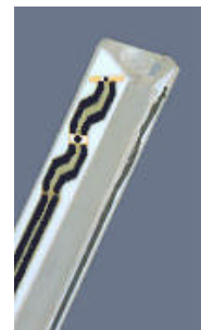
Figure 3.2 Probe Thick-Film Technique
