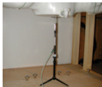
Figure 12.1 Dipole Validation Test Setup
