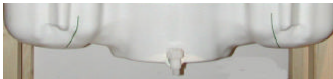
Figure 7.2 SAM Twin Phantom shell
