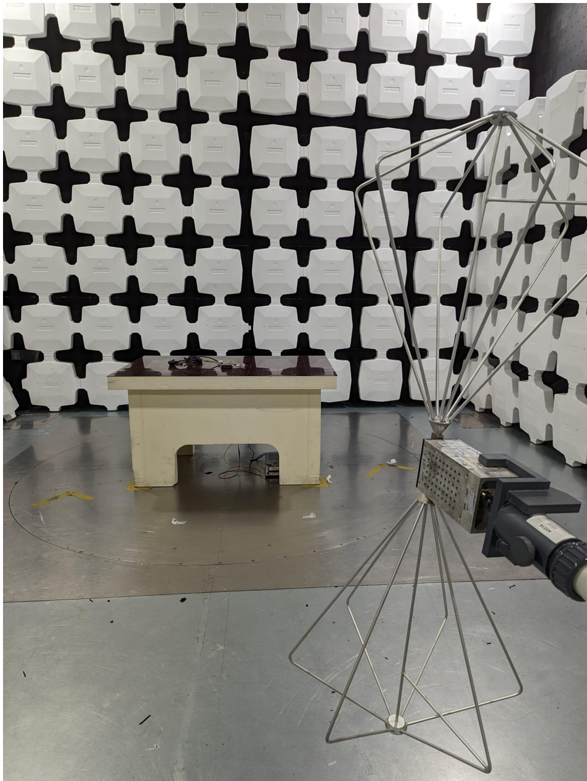
Photo 1 Photograph test setup radiated emissions 30-250 MHz, report section 3.1
