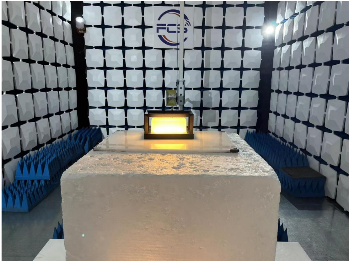
Above 1GHz for radiated emission test setup
