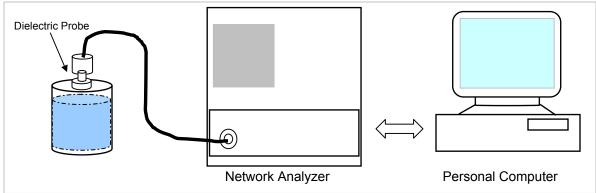
Set-up for liquid parameters check
