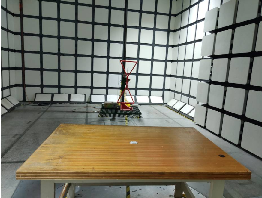
Radiated Emissions View (Below 1 GHz)
