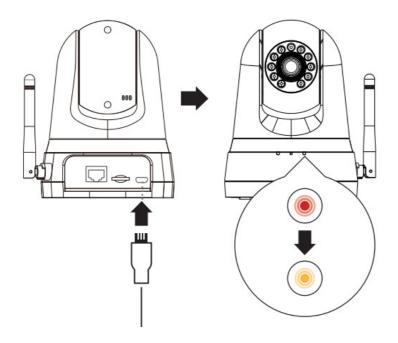
**Wired set-up:** Plug the included USB Power Adapter and Ethernet cable into the back of the camera. Wait until the red PWR LED turns off and the green LINK LED turns on
