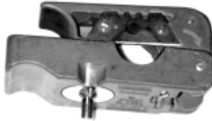
Fig. 8.6-2 Cutter for Assembling 7/8" Feeder Cable Connectors
