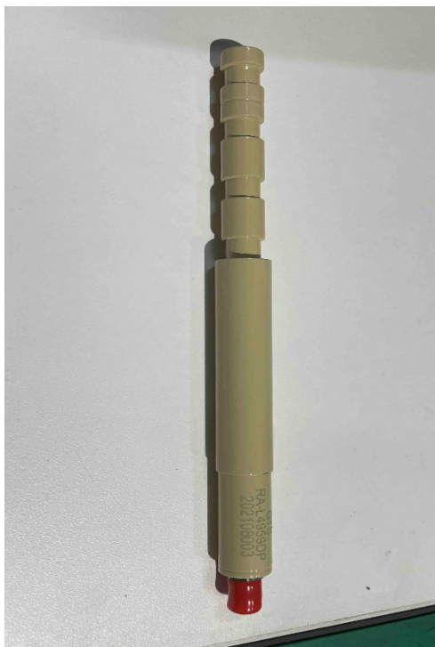
Fig 2 dipole model RA-L4959DP frequency 4900~5900 MHz
