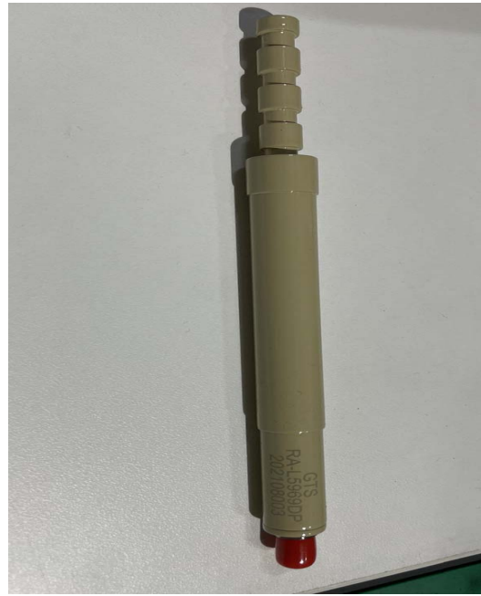
Fig 3 dipole model RA-L5969DP frequency 5900~6900 MHz
