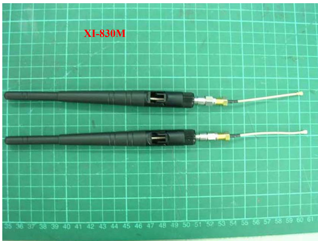
Photo 4: Internal photo of Antenna
