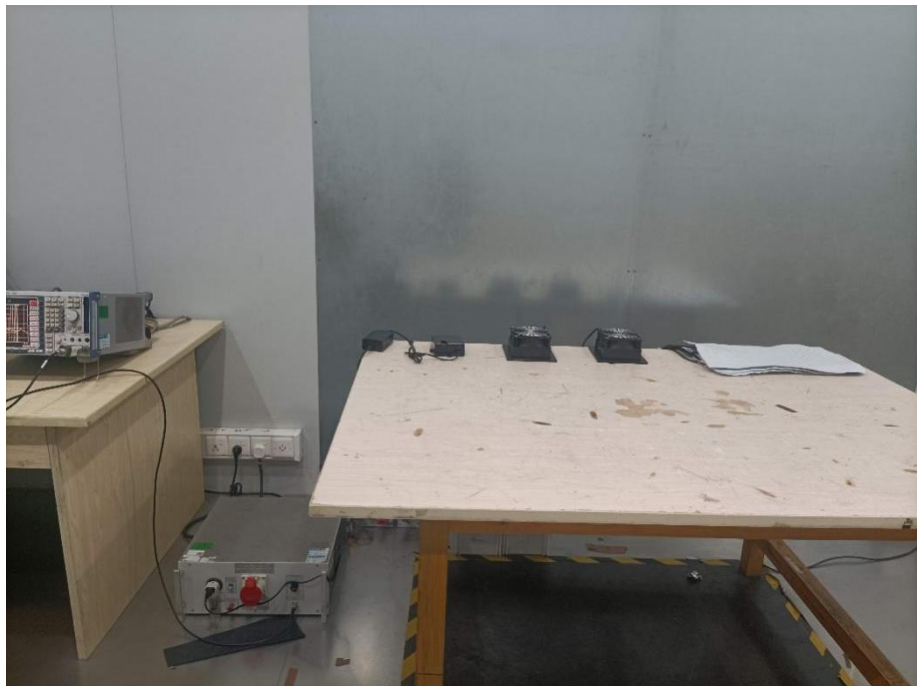
Conducted Emission Test Setup
