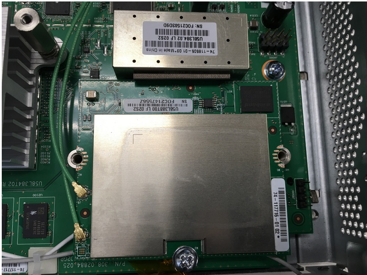
Wifi module without shield
