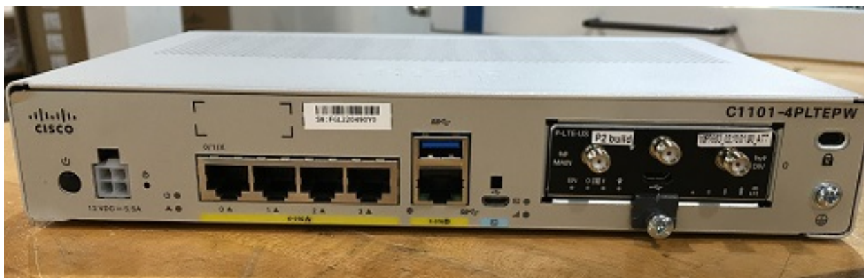
External rear with P-LTE-US module
