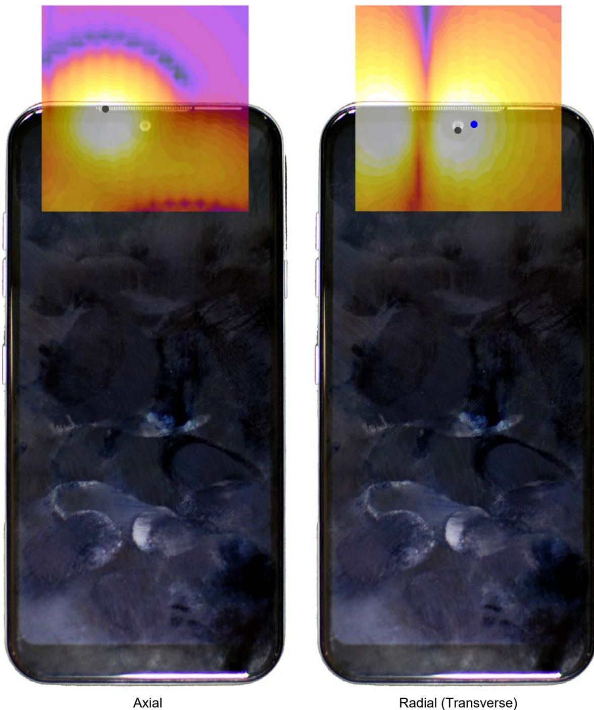
Figure 16-3 T-Coil Scan Overlay Magnetic Field Distributions
