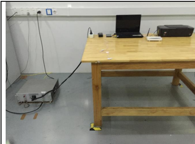
Conducted Emissions Test Setup – Front View
