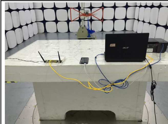
Radiated Emissions Test Setup Below 1GHz
