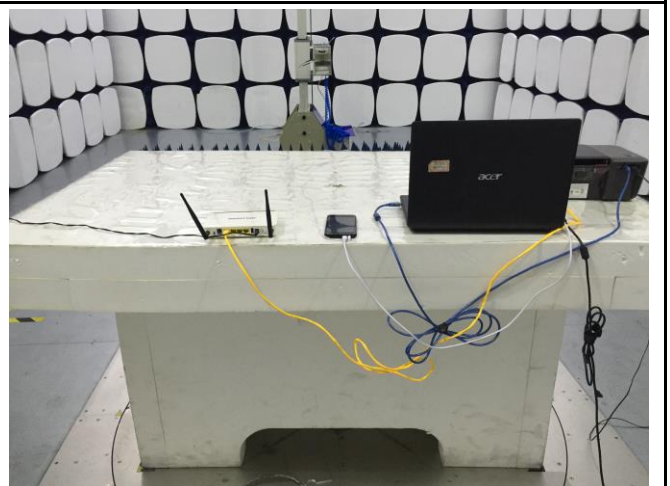
Radiated Emissions Test Setup Above 1GHz
