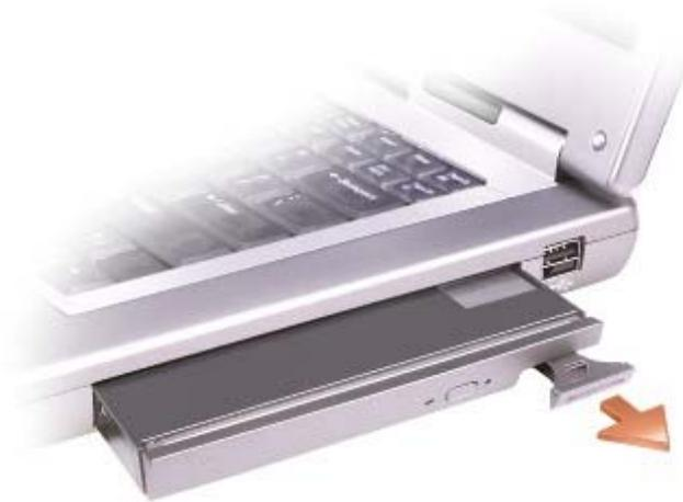
5. Insert the new device into the bay, and push the device until you feel a click.
