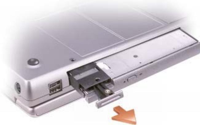
5. Pull the device out of the module bay.
