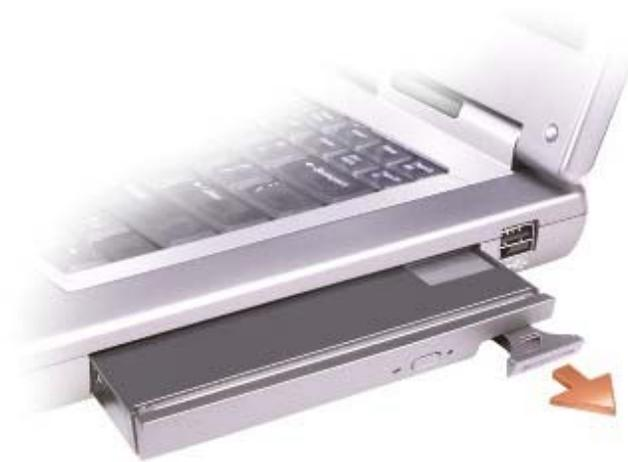
3. Insert the new device into the bay, and push the device until you feel a click.
