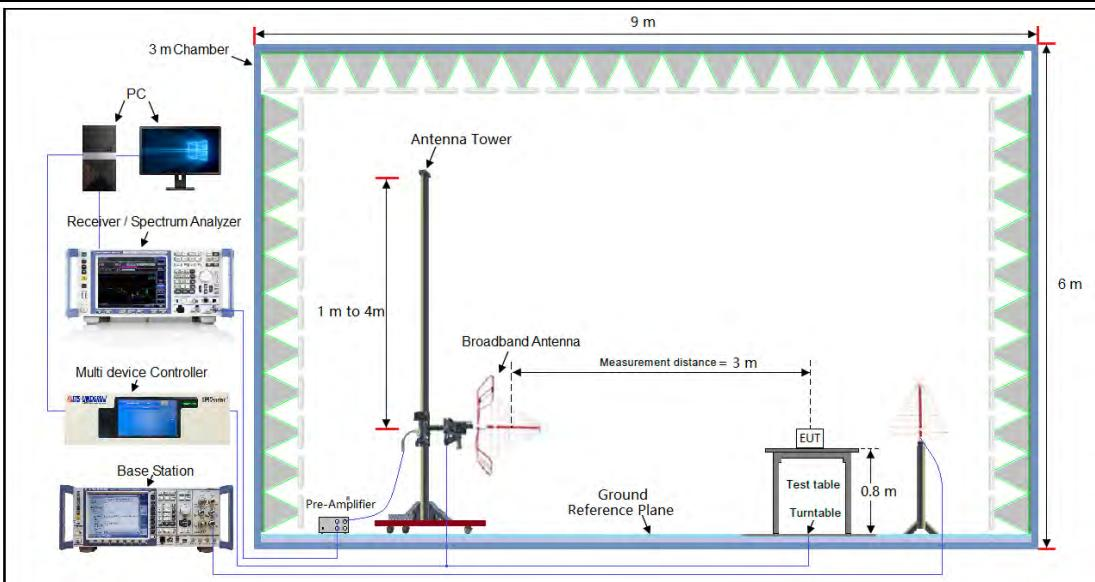
Radiated Emissions Above 1GHz Test setup
