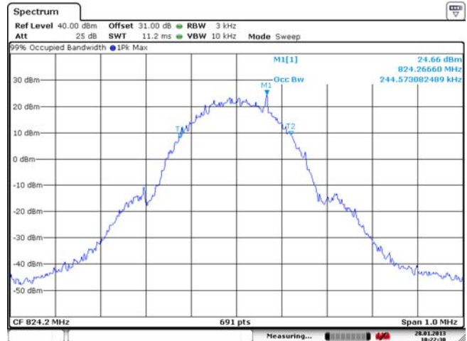
Figure 1-14a: Occupied Bandwidth, GSM850 band Low Channel in GSM mode
