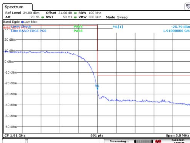
Figure 1-28b: Band 2 High Channel Mask
