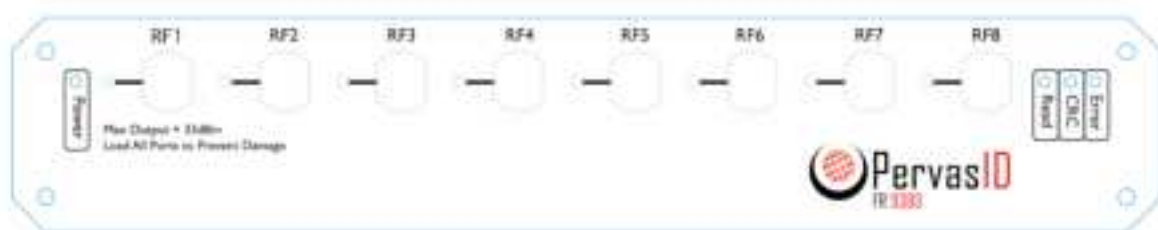
Figure 2: DAS RFID Antenna Ports and Status LEDs
