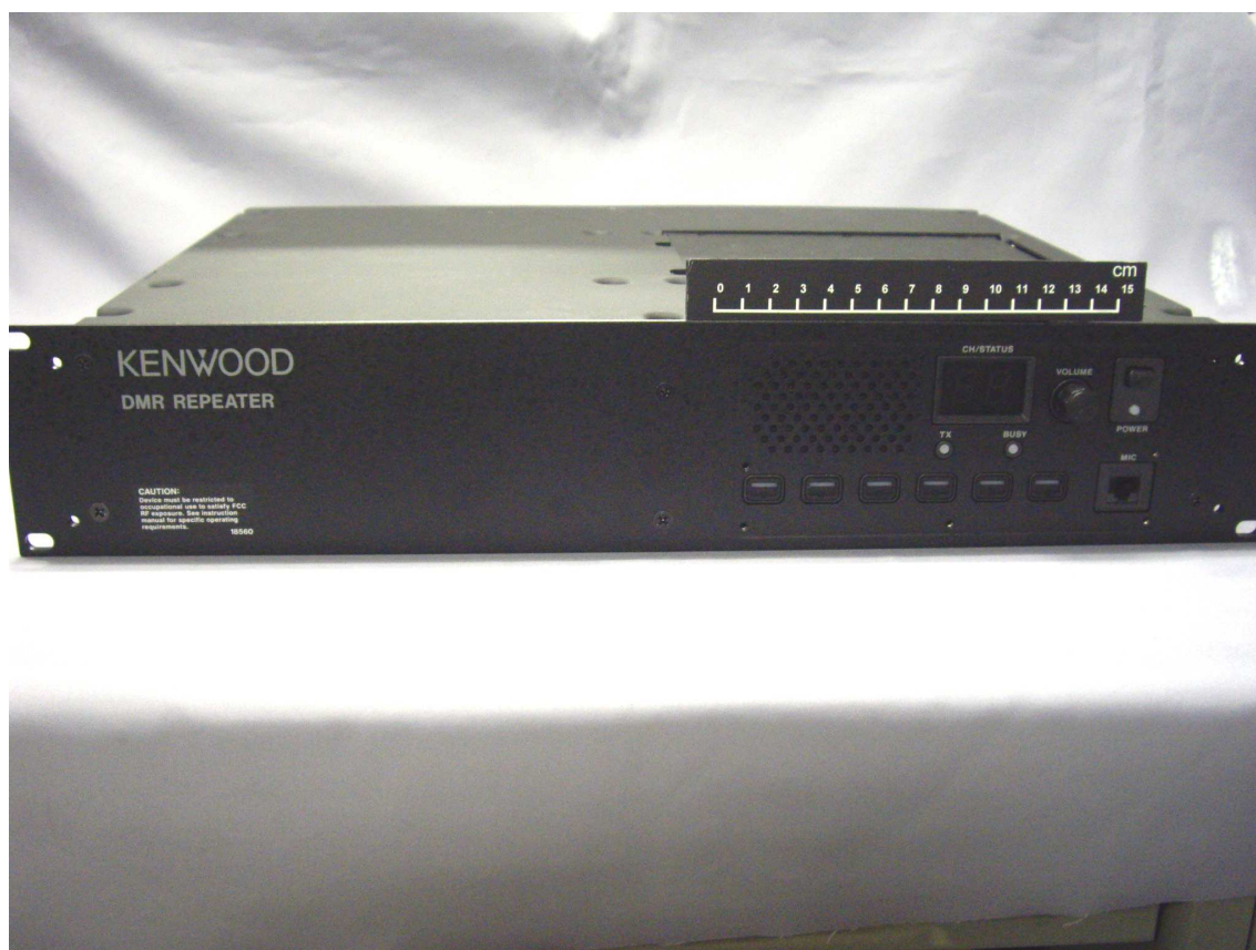
Front View (Caution Label)
