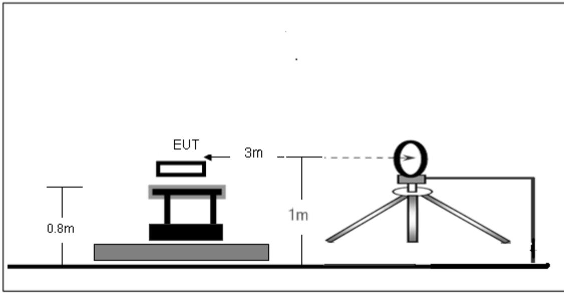
Radiated Emission Test-Up Frequency 30MHz~1GHz
