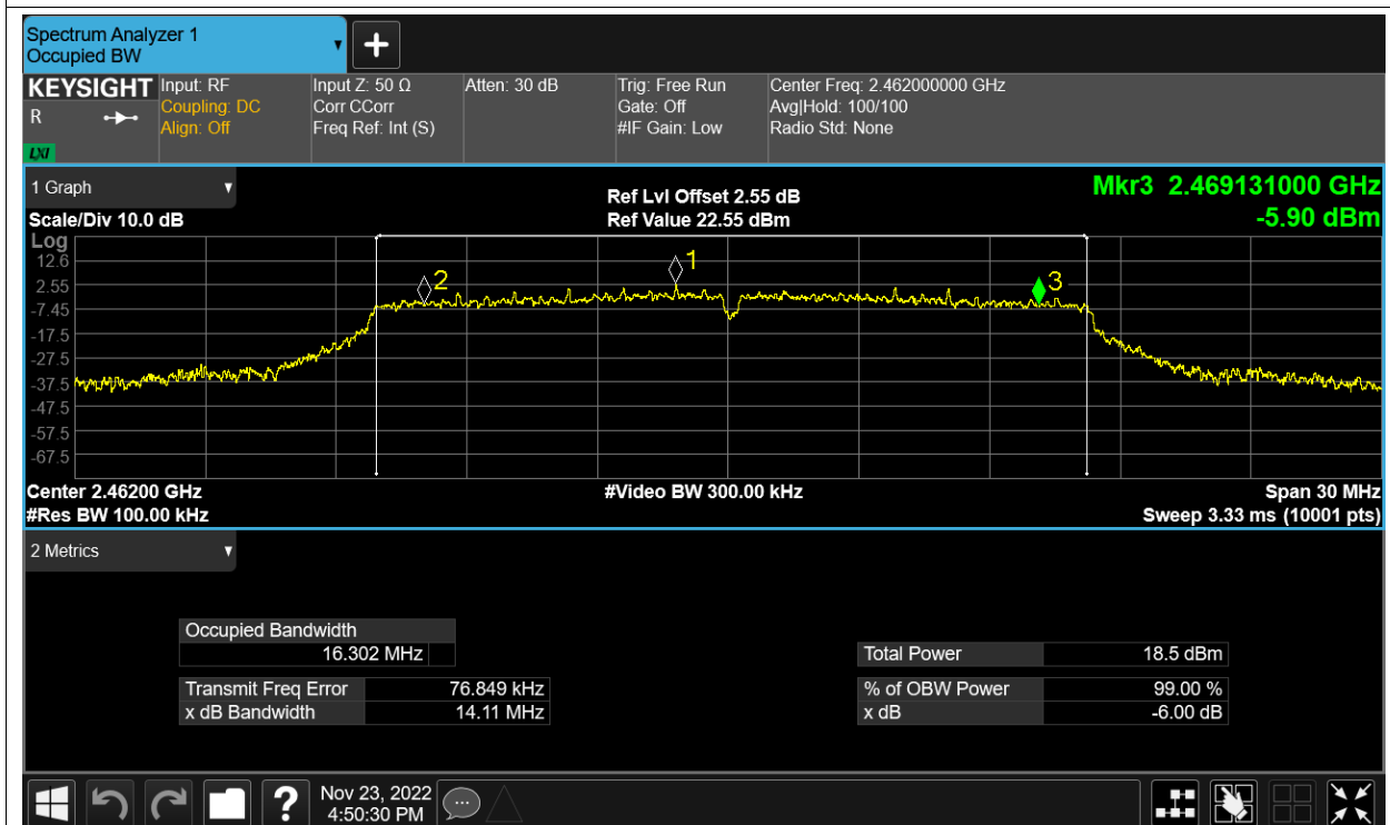
-6dB Bandwidth NVNT n20 2412MHz Ant1
