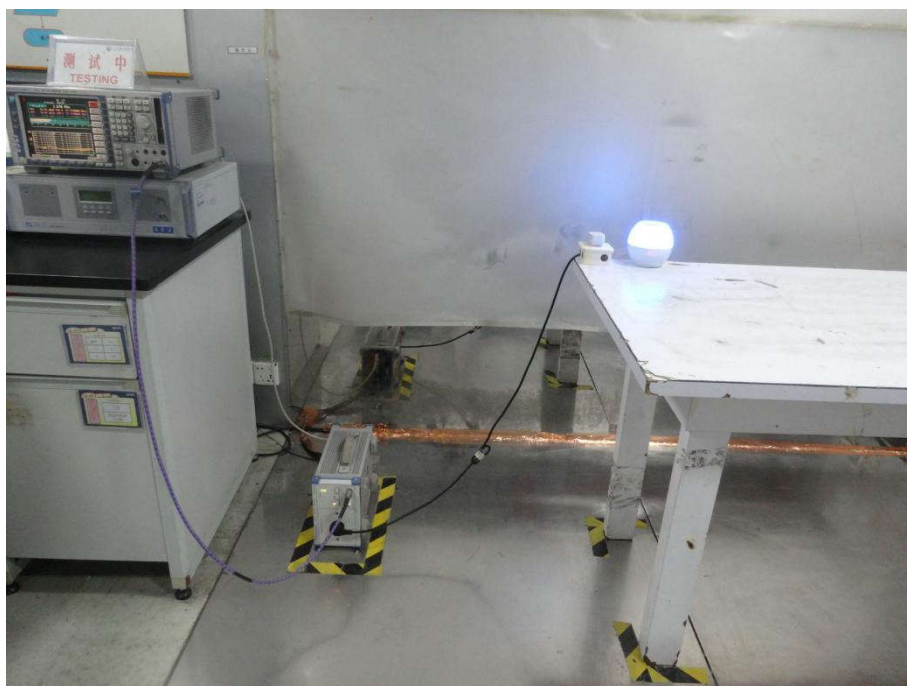
Conducted Emissions Test Setup
