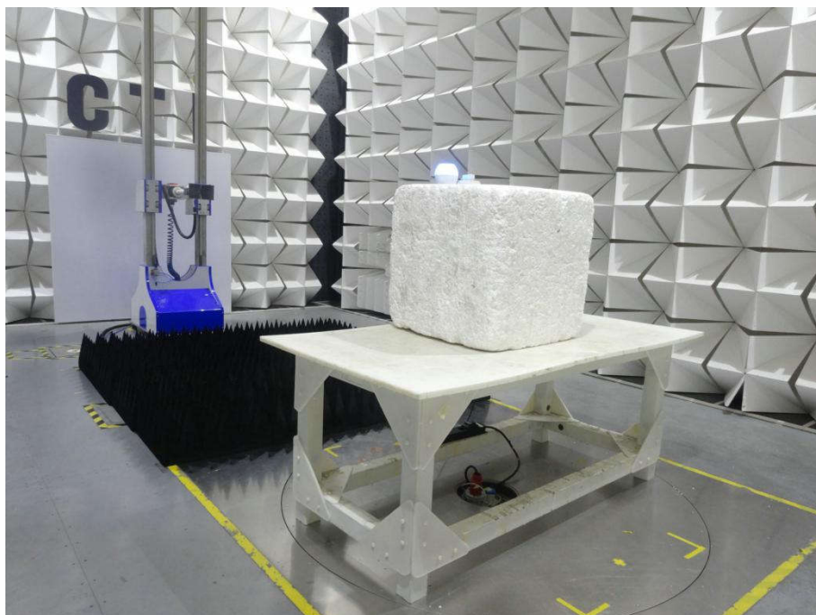
Radiated spurious emission Test Setup-3(Above 1GHz)
