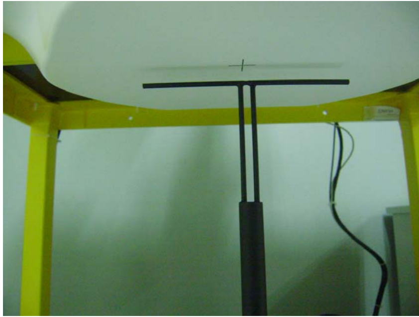
Setup Photo of Dipole Antenna
