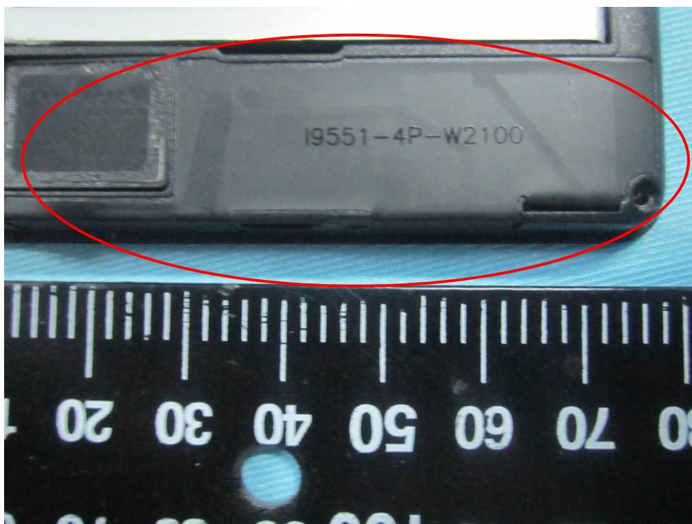
GSM/PCS/UMTS-FDD Antenna View
