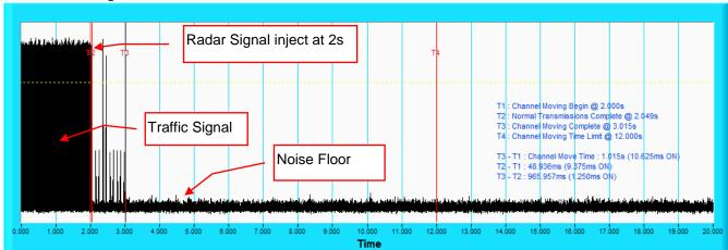
**NOTE:** T1 denotes the start of Channel Move Time upon the end of the last Radar burst at 2s. T2 denotes the data transmission time of 200ms from T1. T4 denotes the 10 second from T1 to observe the aggregate duration of transmissions.
