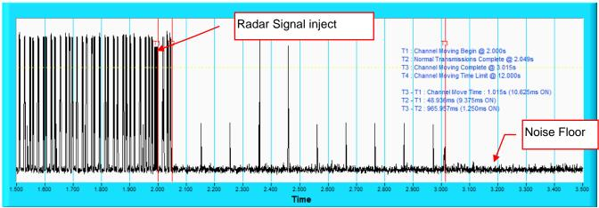
**NOTE:** An expanded plot for the device vacates the channel.
