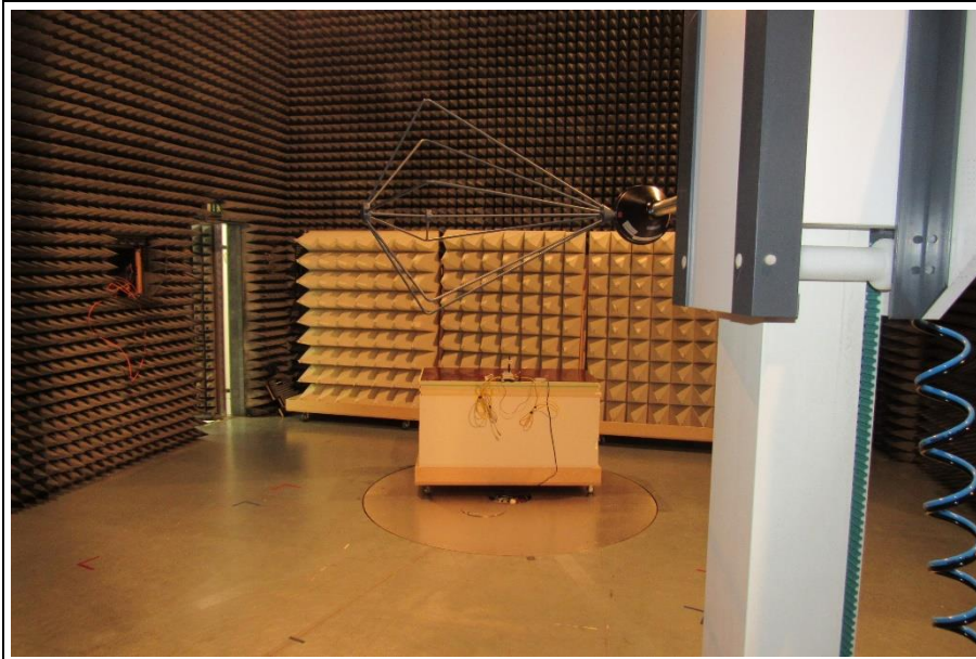
Test setup radiated below 0.2GHz
