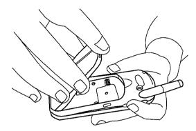
Hold down the top side of the battery. You will hear a click when the battery is secured.
