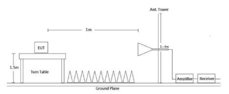
Radiated emission tests were performed in the 3 meters chamber test site, using the setup accordance with the ANSI C63.10-2013. The specification used was the FCC Part 15.209, FCC 15.247 and RSS-Gen, RSS-247 Limits.
