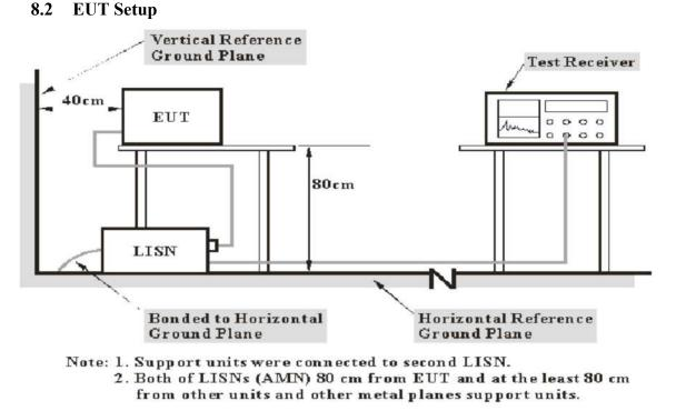
The setup of EUT is according with per ANSI C63.10-2013 measurement procedure. The specification used was with the FCC Part 15.207 and RSS-GEN limits.
